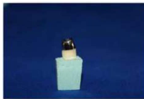
Fig. 2: Coping fabricated by direct metal laser sintering
