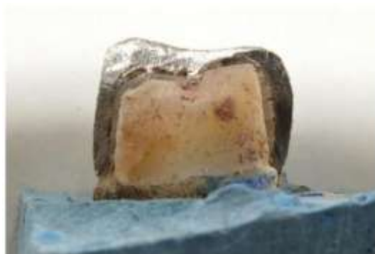
Fig. 7: Microleakage observed in Conventional coping
